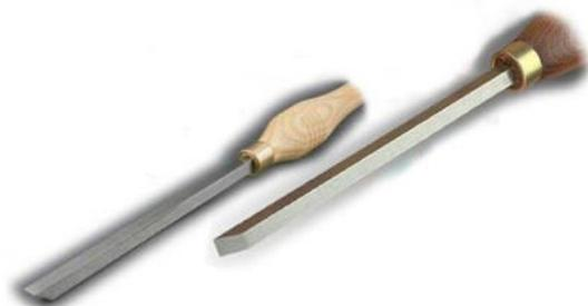
Bedan comes from the French word "bédane" (duck beak). This tool is very old, and was used for turning long before gouges appeared. The bedan is a rectangle often square (sometimes trapezoidal) with one bevel of about 45 degrees. They are commonly used for spindle turning, and are often used when turning trembleurs. With care they can also be used for hollowing and scraping. A bedan can be used like a
