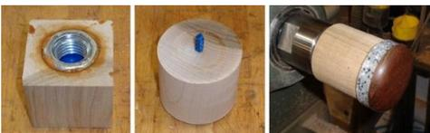
the spindle, drill a second hole at the bottom of the first hole deep enough so the spindle will not bottom out. Next, glue the nut into the hole making the nut as square to the wood as possible (epoxy is good). A piece of tape over each end of the nut will keep glue away from the threads. When the glue has set, put it on the lathe, turn off the corners, and true-up the face. The “Nut Chuck” can now be used in any way you like.
