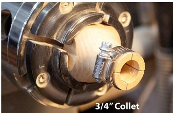
You can make a quick collet chuck with a block of wood and a hose clamp. Turn the block round and make a tenon for a four-jaw chuck. Drill a hole to match the piece you want to hold. Cut a shallow channel near the end to hold and guide the hose clamp. Now with a
