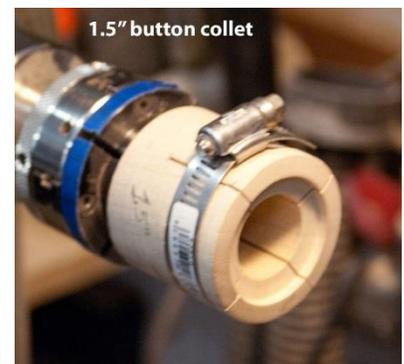
saw make two cuts to about the depth of the drilled hole. (A wider kerf will allow for more adjustment.) You now have a custom collet chuck. A small hose clamp can be used as a height stop for your tool rest. This can save a little time when you have to change the angle of the tool rest often for a project. When
