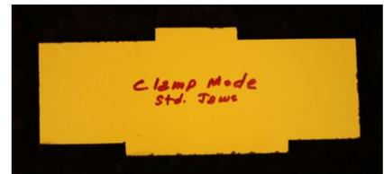
Now make another gauge for the compression mode of your chuck. It is a good idea to mark each gauge for its intended use, e.g., Vicmarc 5 1/2" expansion mode. If you change jaws in your chuck, it is easy to make gauges for each set of jaws.
