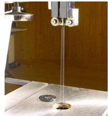
Use this method each time you change blades, and remember to de-tension the blade with the quick-release tensioner when not in use. (If your bandsaw doesn't have a quick-release lever, make it a habit to relax the tension by a specific number of turns — 10, for example — at the end of each day you use the saw. Next time you need the saw, just tighten the wheel 10 turns to return to the correct tension.) — From the Editors of Wood Magazine at [WoodMagazine.com](http://WoodMagazine.com)
