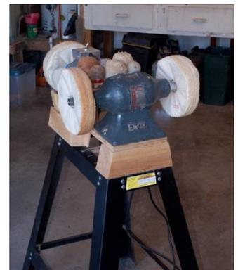
the shaft for maximum clearance. I got a tool stand from Harbor Freight (\$34.95) and with a little woodwork, I built a riser to mount the grinder on one end and the old motor on the other. I added pockets to hold the buffing compounds and a place to hold the buffing balls. It saves time and keeps everything in one place so the Old Greek can't hide them. Now where did he hide my camera? – John Nikakis
