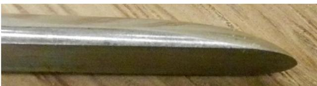
Grind a 30 to 35 degree convex cutting edge to the rounded end of the flat area.
