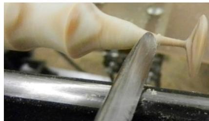
Even softer fir can be turned to toothpick size with the lightest touch and no support.
