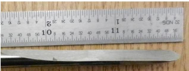
Grind two inches of the end of the rod flat to 1/8" thick. Two inches of flat provides for years of sharpening.
