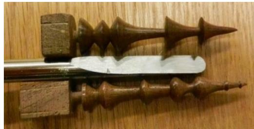
3/8" square stock with the feather touch fluteless gouge. The lower one is walnut, which usually does not make good small finials with fine detail. The harder fine grain wood on top allows for more detail. These spindles were both turned unsupported and are about three inches long.
