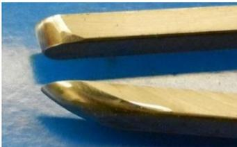
Top is 80 degrees. Bottom is 35 degrees. These are 1/2"x1/4" steel scrapers, top standard, bottom remade into gouge.
