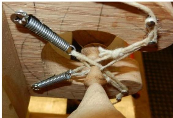
In this example, the rest is positioned close to the cup of the goblet.
