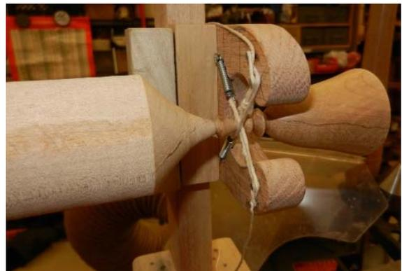
“X” with a single string from a nail to each spring. The center is put around the neck of the goblet and a second string from each spring goes over the other side of the neck and around the nail while keeping tension on the spring and tying off using the other nail. This can be seen clearly in the overhead shots.
