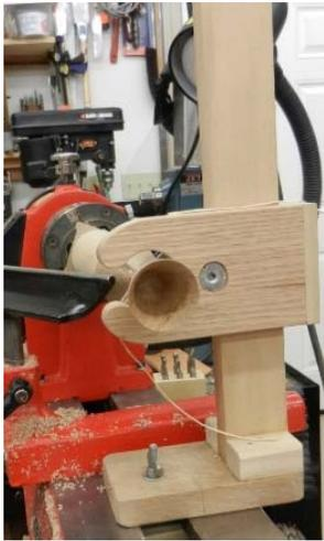
Depending on the length of the turning, several string steadies can be used on longer pieces and can be added as you complete each section. Since these steadies are generally shop made, the cost is small. You can add as many as you like.
