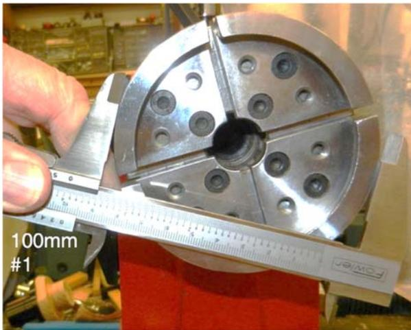
The Super Nova chuck comes standard with 50mm jaws. 100mm jaws are available. 50mm is approximately 2" in diameter which is a circumference of about 6.28". 100mm is approximately 4" in diameter which is a circumference of about 12.65". A 1-pound force of the chuck is doubled with 100mm jaws over 50mm jaws. This only happens when the 100mm jaws are set at 100mm. The jaws form a circle at 100mm as seen in #1.
