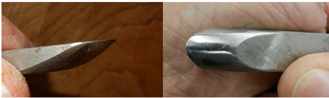
This shows the grind which makes it easier to enter the cut cleanly.
