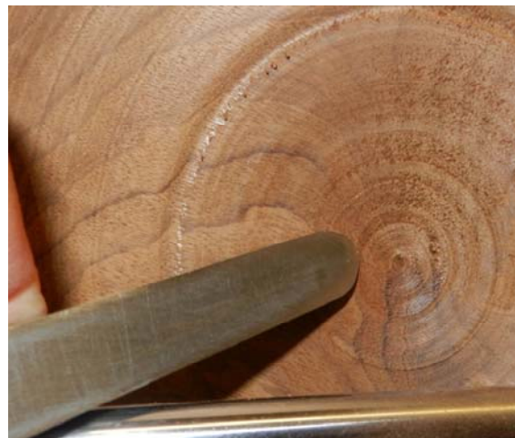
This shows the grind which makes it easier to enter the cut cleanly.
