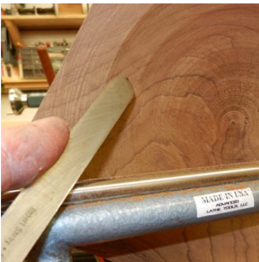
This shows the grind which makes it easier to enter the cut cleanly.
