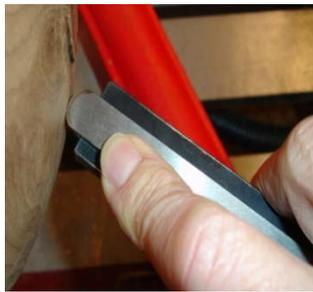
more stable way to cut with this type of grind is a "box tool rest". (The box rest is black and directly under the tool.) There are several types of these designed to go inside of boxes and bowls, but they also offer the best support and work great on the outside of projects. They give great tool control and produce a superior finish.
