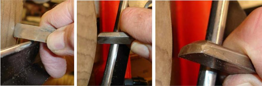
The middle picture to the left shows the tool is riding on the bevel which is about 10 degrees and at a compound angle to the workpiece. The direction of the cut is toward the left of the tool rest. This is a light cut and will produce very fine shavings. I
