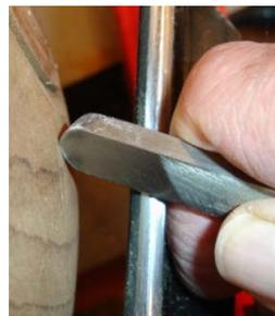
In the right-hand picture to the left you can see the pull cut and the grain direction of the wood does matter. Cut with the grain for the least tear out. The diagram illustrates tool position.
