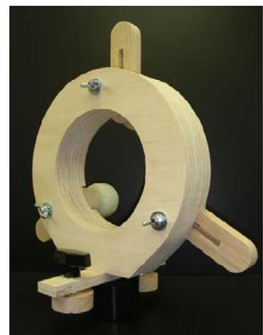
To ensure precise alignment of the slot in the arm and the ring slot bolt hole, I completed construction of the arms first, then used a transfer punch through the arm slot to mark the hole location in the ring slots.
