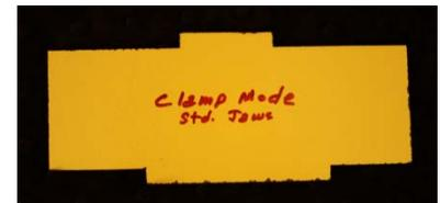
Now make another gauge for the compression mode of your chuck. It is a good idea to mark each gauge for its intended use, e.g., Vicmarc 5 1/2" expansion mode. If you change jaws in your chuck, it is easy to make gauges for each set of jaws.
