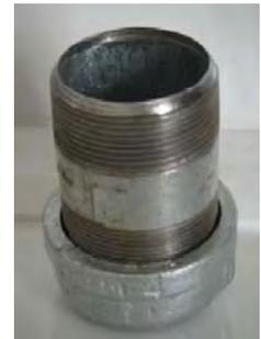
To cut the discs, lay the roll stock flat on a block of wood, put the cutting edge in a position to yield the most discs, and hit the cap with a heavy hammer. A 4-pound sledge worked best for me. – Bill Draper
