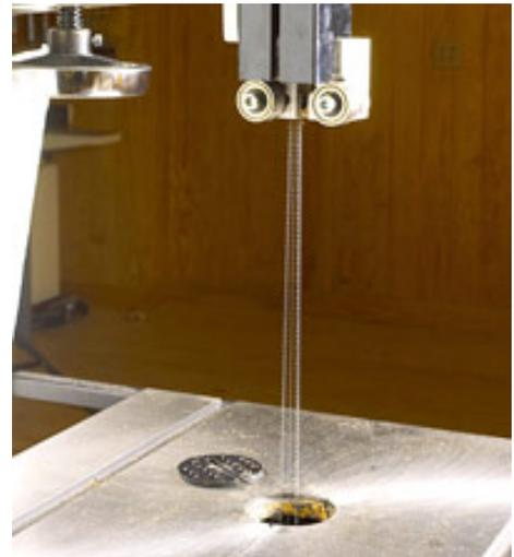
Use this method each time you change blades, and remember to de-tension the blade with the quick-release tensioner when not in use. (If your bandsaw doesn't have a quick-release lever, make it a habit to relax the tension by a specific number of turns — 10, for example — at the end of each day you use the saw. Next time you need the saw, just tighten the wheel 10 turns to return to the correct tension.) – from the Editors of Wood Magazine at [WoodMagazine.com](http://WoodMagazine.com)
